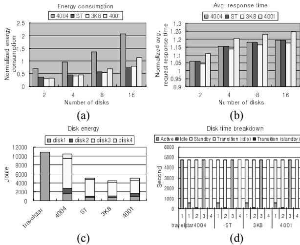
**Figure 3. (a) energy consumption and (b) avg. request response time of smaller disks varying the number of disks. (c) energy distribution and (d) disk time breakdown when four disks are used for each disk type.**
