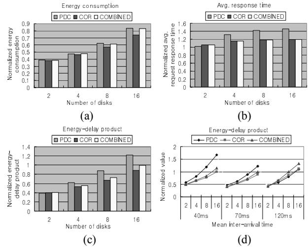
**Figure 4. (a) energy consumption, (b) avg. request response time, and (c) energy-delay product of each file placement technique varying the number of disks. (d) energy-delay product according to a different mean inter-arrival time.**
