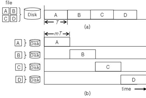
**Figure 1. File access behaviors of a 2.5" disk and multiple smaller disks under the perfect file placement**
