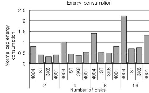
**Figure 2. Normalized energy consumption of smaller disks varying the number of disks**
